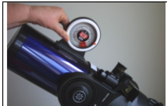
Figure 10. Use protractor to check OTA to latitude. Verifies declination circle setting.
