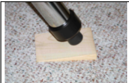
Figure 6. Tapered leveling block for fixed length tripod legs.
