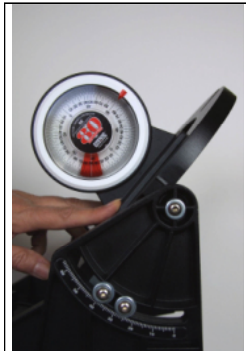
Figure 7. Use protractor to adjust wedge for latitude.
