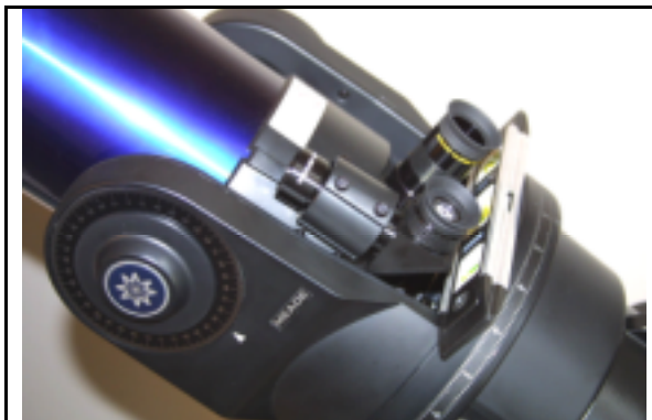
Figure 9. Final leveling of forks using the torpedo level.
