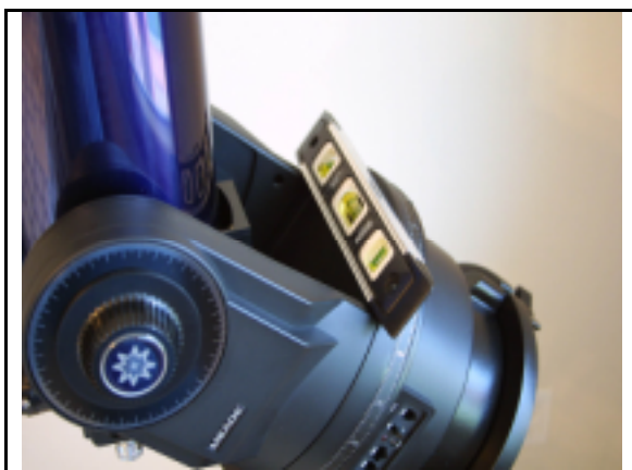
Figure 8. Position of torpedo level across OTA forks
